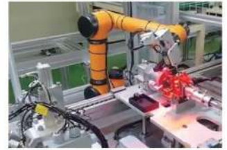
Appearance inspection of auto parts
